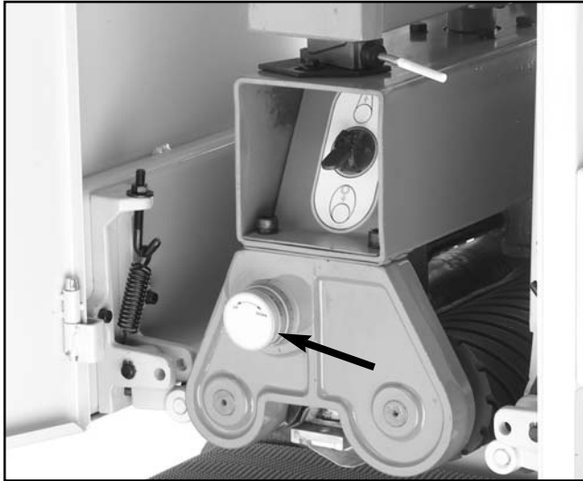
Figure 17. The scale on this knob tells you how far you have moved the platen.
